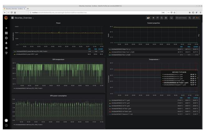
Fig. 2. Typical Grafana view of the monitoring results in a web brouser
